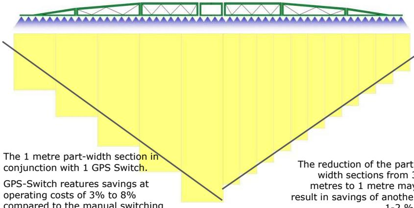
The 1 metre part-width section in conjunction with 1 GPS Switch.
