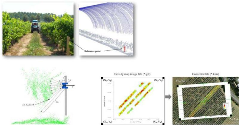
Ultrasonic and LIDAR Sensors for Electronic Canopy Characterization in Vineyards: Advances to Improve Pesticide: Application Methods *Sensors* 2011, 11, 2177-2194; doi:10.3390/s110202177
