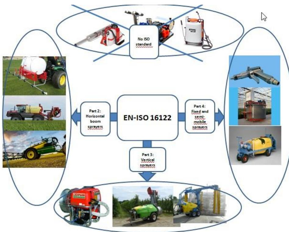
In the EN-ISO 16122 part 1 are defined the general requirements to be fulfilled, a classification of sprayers in order to define to application of each part of EN-ISO16122 and also the minimum requirements for the preparation of the sprayer including the minimum safety requirements dealing with operator safety during the inspection.
