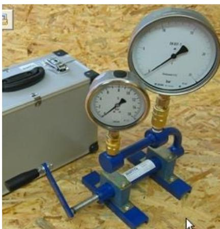
Measurements shall be carried out with both increasing and decreasing pressure. In any case accuracy of the pressure indicator shall be checked at minimum of four equally points within the relevant working pressure range. The pressure shall be stable during measurement, example no influence from pump rotations and pulsations. The test be made within a working pressure range suitable for the nozzles mounted on the sprayer under test.
