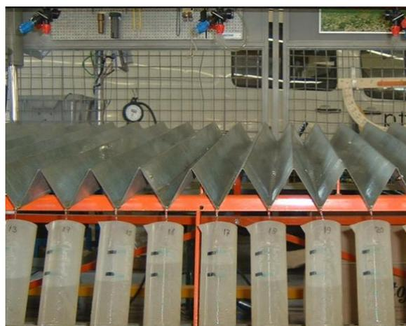
When using a mechanical groove patternator the Coefficient of Variation (CV) has to be calculated with this formula:
