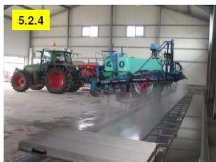
The groove width of patternator working in steps with electronic data sampling (e.g. scanners) shall correspond to the mentioned dimensions. The tolerance is  $\pm 1$  mm. When passing the measuring track, the positioning in the single steps shall be completed with an accuracy of  $\pm 20$  mm. The measuring error of the flow volume of the single grooves at a flow volume of 300 ml/min shall be less than 4 %. The instruction handbook shall give information on how to adjust the patternator.
