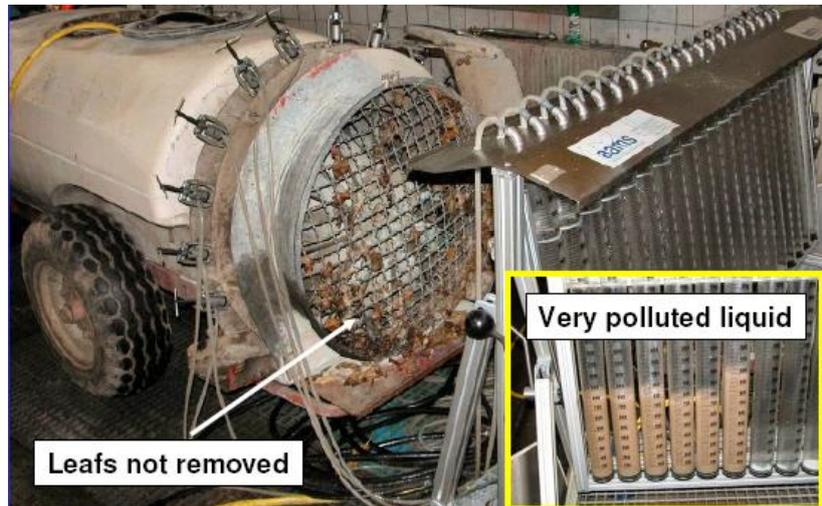
Special attention has to be paid to rinsing and internal cleaning of the sprayer including filters and filter inserts, and external cleaning of those parts of the sprayer that are most exposed to the crop protection products when spraying.
